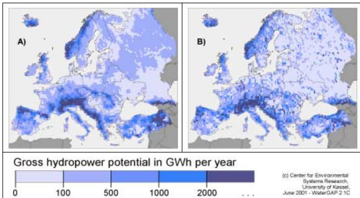
**Figure 8.1:** Gross hydropower potentials for Europe, calculated by applying average (1961-90) runoff and discharge values of WaterGAP 2.1. A) Each cell is assigned its total gross hydropower potential down to sea level. B) Only the portion of the gross hydropower potential that can be locally utilized down to the next downstream cell is allocated to each cell.
