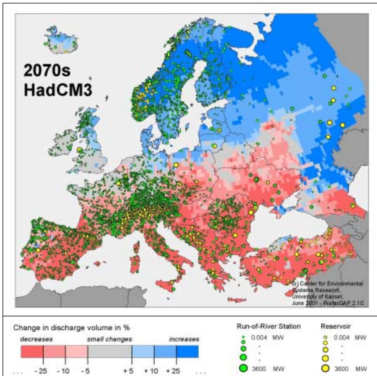
**Figure 8.2:** Relative change of average (1961-90) total discharge volumes calculated with WaterGAP 2.1 for the 2070s (HadCM3 climate model and Baseline-A water use scenario), superimposed by geo-referenced European hydropower plants, classified according to their type and capacity.
