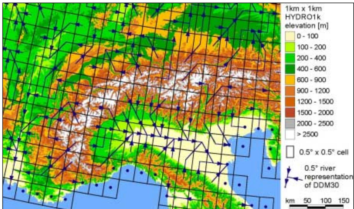
**Figure 8.4:** A grid of 0.5° x 0.5° cells and the DDM30 drainage directions as applied in the WaterGAP model superimposed on the HYDRO1k digital elevation model.
